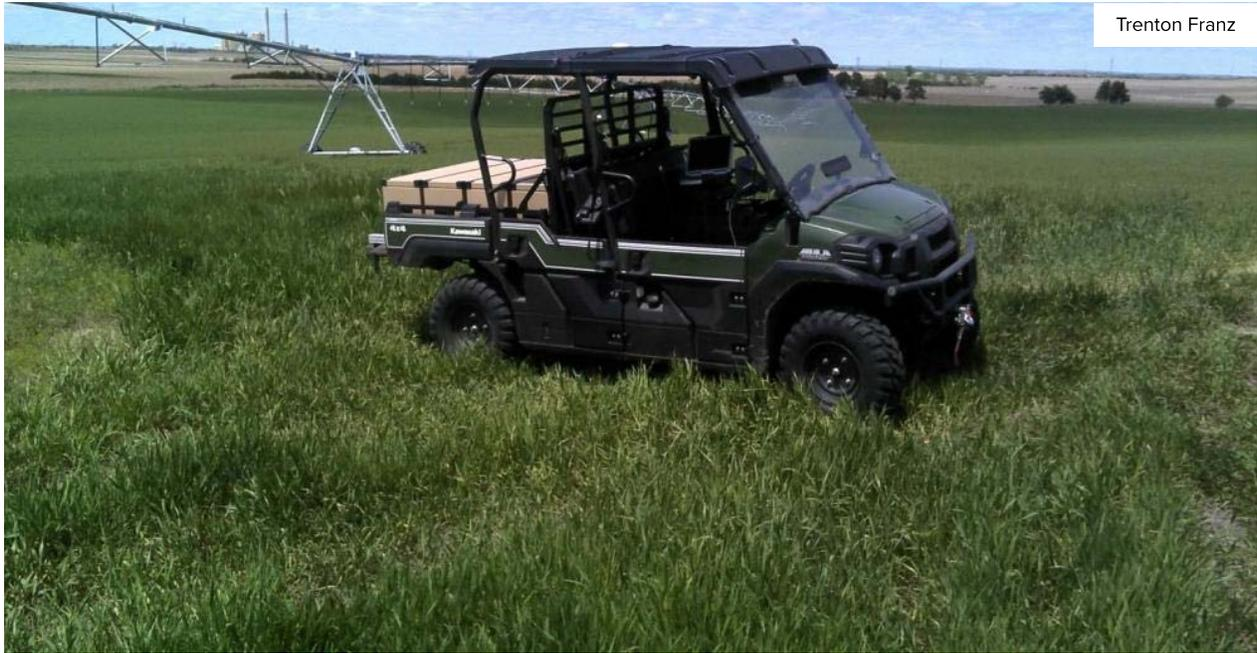
*FARMER-FRIENDLY: A Cosmic ray neutron probe on Roric Paulman's farm is mounted on an all-terrain vehicle to take measurements every minute. Using the mobile unit, a quarter section can be mapped in as little as 60 minutes.*
